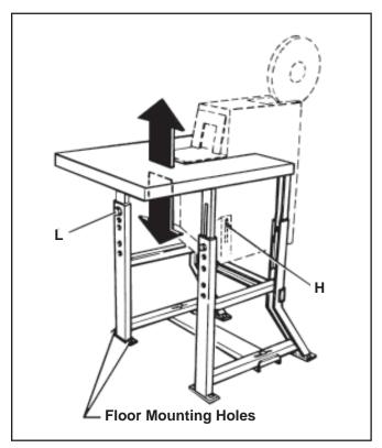
Figure 14-2 Work Surface Adjustment - Right Front View
