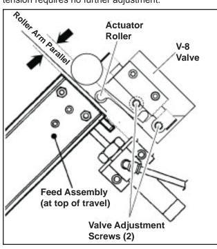
Figure 8-1 V-8 Valve Adjustment
