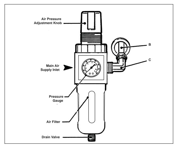
Figure 5-4 Air Control Unit – Set-Up
