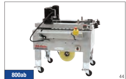
800ab 3M-Matic™ Case Sealer 800ab is an adjustable side belt drive case sealer. Applies bottom seal only at rates up to 40 cases per minute, using tape widths from 36mm to 48mm, and also 72mm tape.
