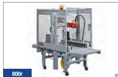
800r 49 3M-Matic™ Case Sealer 800r is a semi-automatic random case sealer automatically adjusts for case height and width. Top and bottom seal at rates up to 20 cases per minute, using tape widths from 36mm to 48mm wide.
