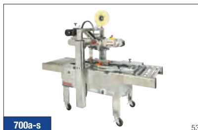
700a-s 53 3M-Matic™ Adjustable Case Sealer 700a-s stainless steel has advanced features to seal uniform cases up to 30 per minute. Dual masts with dual lead screws for stability and uniform height adjustments. Adjustable top and bottom belt drive system for reliable conveyance of heavier or tall/light boxes. Compression rollers position each box for precise tape sealing. Stainless construction for corrosive environments.
