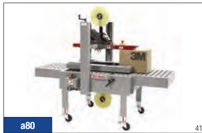
a80 3M-Matic™ Adjustable Case Sealer a80 is an adjustable side belt drive case sealer that dependably seals uniform size cases.
