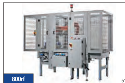
800rf 51 3M-Matic™ Case Sealer 800rf Type 40800 is a fully automatic random size case sealer that automatically adjusts for various case sizes and folds the top minor and major flaps up to 10 cases per minute. Using tape widths from 36mm to 48mm tape widths.
