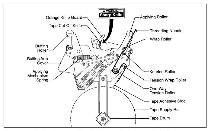
Figure 3-2 - Taping Head Components/Threading Diagram - Lower Head (Left Side View)
