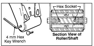
Figure 4-3 – Section View of Roller Shaft
