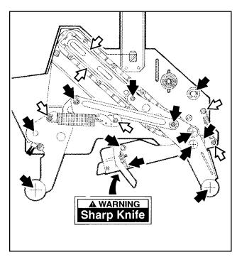
Figure 4-2 – Lubrication Points, Upper and Lower Taping Heads
