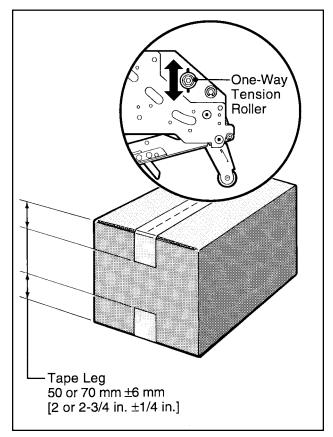
Figure 5-5 - Leading Tape Leg Length
