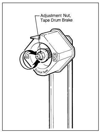
Figure 5-2 - Tape Drum Friction Brake
