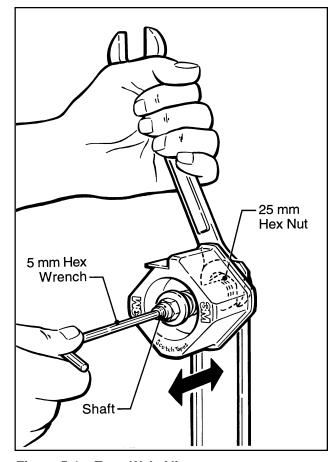
Figure 5-1 – Tape Web Alignment
