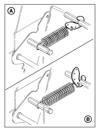
Figure 5-3 – Applying Mechanism Spring
