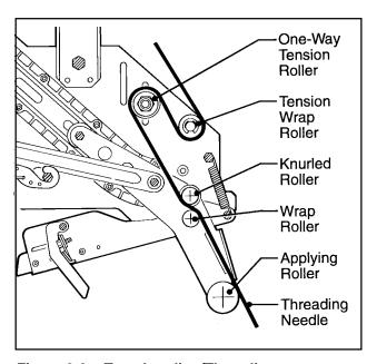
Figure 3-3 - Tape Loading/Threading
