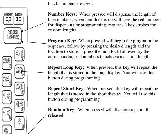
**TD2100 PREMIUM Keypad** - The Premium keypad offers all the same function as the STANDARD keypad plus it is possible for you to dispense any length of tape from 5" to 99" in 1" increments. The exception from the STANDARD keypad is there are 10 preset lengths versus 20. There are two versions of the PREMIUM keypad, Short and Long. The Long version has longer pre-programmed lengths than the Short.
