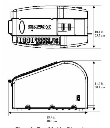
**Figure 1 – Tape Machine Dimensions**
