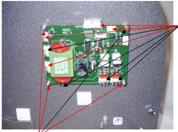
3. Remove the screws from the controller board.
