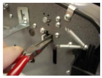
4. Remove the fixed blade using the same pair of needle-nose pliers.
