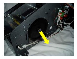
5. Remove the large timing pulley from the feed wheel shaft.
