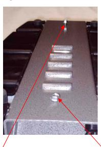
Loosen both screws on the bottom of the chassis.
