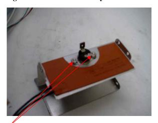
5. With one hand holding a screw driver inside the water tank holder, remove the nuts holding on the thermostat.
