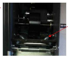
This is how the solenoid spring should look once the tape channel plate is removed (refer to Removing the Tape Channel Plate [p. 34]).
