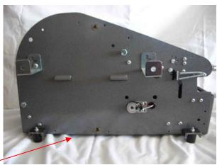
4. Slide the left side cover towards the bottom of the machine and pull the left side cover away.
