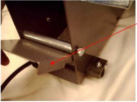
6. Attach the four screws to the new ramp inside the machine so that the thicker end of the ramp is toward the rear of the machine.
