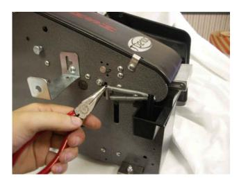
3. Use a pair of need-nose pliers to remove the springs that are attached to the blade shoe.
