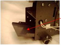
7. With one hand pushing the chassis slightly apart, position the new front cover.
