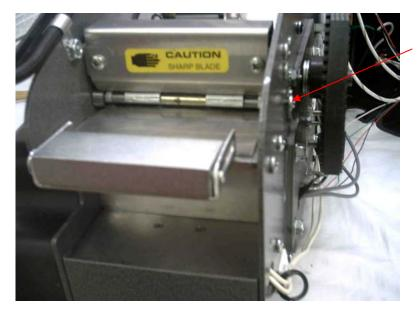
5. Remove the screws from the flapper shaft.
