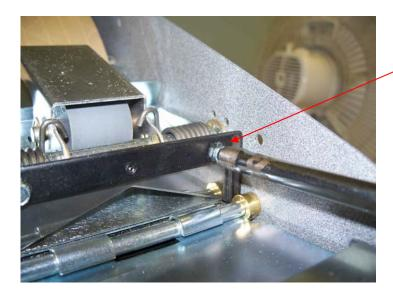
4. Remove the two remaining screws and lift the moveable cutter blade out of the machine.
