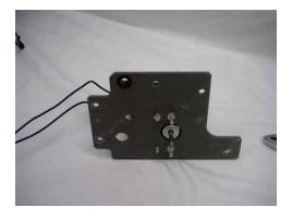
12. Remove all the electrical connections from the gearbox/motor mount.
