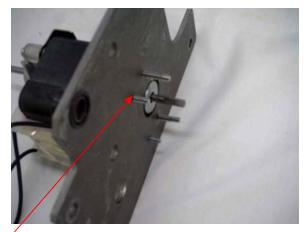
10. Place the new motor onto the gearbox/motor mount.
