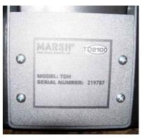
1. Remove the screws on the front of the machine and the cover will be removable.
