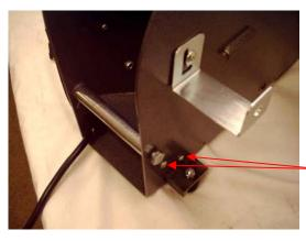
4. Remove the four screws holding the ramp in and remove the ramp.
