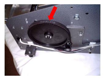
3. Facing the right side of the machine, remove the timing belt from the large timing pulley first, then from the small timing pulley.
