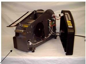
6. Remove the three screws along the outside of the machine.
