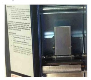
2. Remove the pressure plate.
