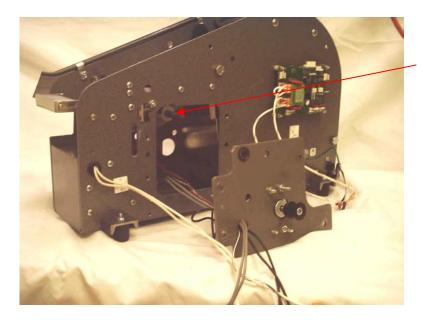
7. Remove the feed wheel shaft and the feed wheel from the chassis at a downward angle.
