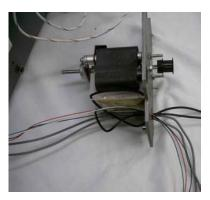
11. Pull the gearbox/motor mount assembly out of the machine.
