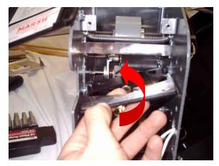
13. Twist the movable cutter assembly and remove from the machine.
