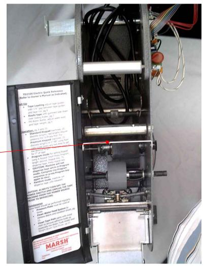
1. Insert the tape basket/motor cover into the machine going straight through the top and middle of the machine.
