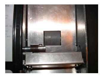
4. With the left end of the pinch roller spring on top of the screw on the left side of the machine, slide the pinch roller shaft into the right side of the chassis.
