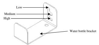
Figure 5 – Adjustable Water Level Positions
