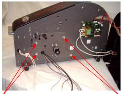
10. Remove the four large screws from the gearbox/motor mount.
