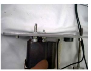
13. Looking at the outside surface of the gearbox/motor mount, attach the screws that are on the left hand side of the gearbox/motor mount tightly and the nuts on the right snugly
