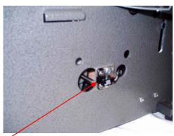
9. With one hand holding the encoder wheel, remove the screw holding encoder wheel.
