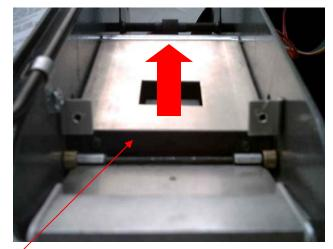
10. Push down on the movable cutter assembly, then pull up on the tape channel plate so that the tape channel plate and the dead roller rotate so that the screws underneath
