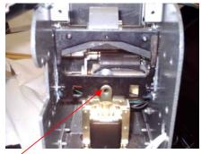
11. Remove the screw holding the movable cutter to the solenoid.
