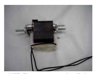
NOTE: The motor is square when all of the plastic is touching the gearbox/motor mount.
