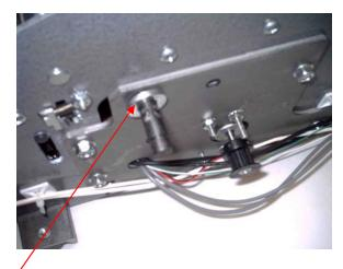
NOTE: Make sure that any washers that were on the feed wheel shaft are now placed back on the feed wheel shaft.
