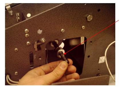
9. Insert the new feed wheel shaft and feed wheel into the chassis into the bearing.
