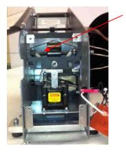
10. Remove the solenoid spring from the shoulder bolt connecting it from the solenoid.
