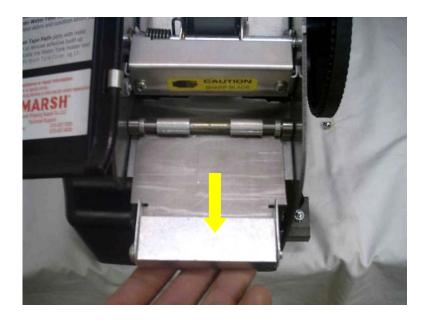
6. Slide the flapper shaft, weighted brush cover, tape weight, and bushings from the front of the machine.
