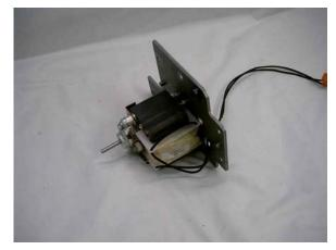
9. Pull the motor electrical connections through the gearbox/motor mount.
