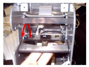
12. Rotate the movable cutter assembly towards the front of the machine.
