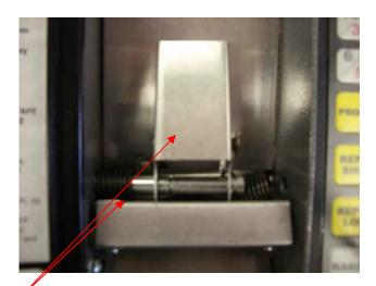
6. With one hand holding the pinch roller and the pinch roller spring, slide the pinch roller shaft to the left till the pinch roller shaft is no longer on the chassis.
