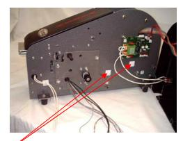
8. Set the HEATER connector off to the side.
