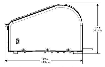
**Figure 1 - Tape Machine Dimensions**
