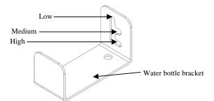
Figure 5 – Adjustable Water Level Positions
