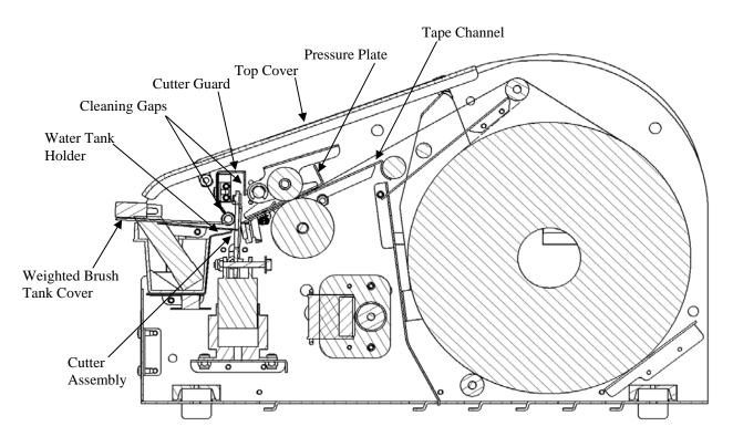
Figure 9 – Cleaning the Cutter Assembly, Cleaning the Tape Path
