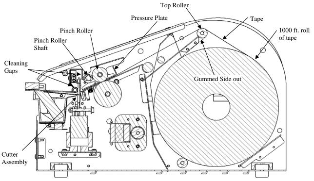
Figure 3 – Tape Routing
