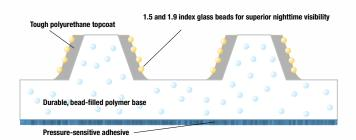
This cross-section of 3M™ Stamark™ Tape Series 270 shows how 3M's advanced technologies make this tape a durable value for intersection safety.
