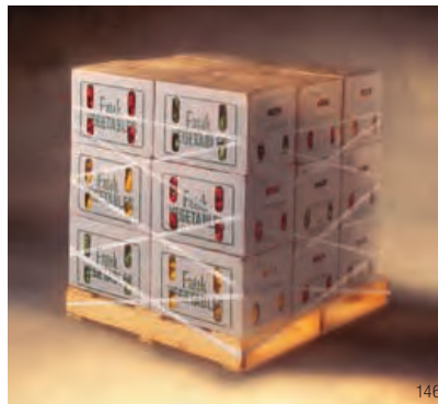
“X”-pattern can contain loads for shipment anywhere.
