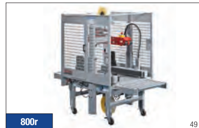
800r 49 3M-Matic™ Case Sealer 800r is a semi-automatic random case sealer automatically adjusts for case height and width. Top and bottom seal at rates up to 20 cases per minute, using tape widths from 36mm to 48mm wide.
